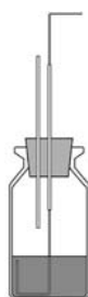
Fig. 3 The ampoule in which the experiments were performed. The rubber stopper was fitted with steel tubes to make mixing of cement and water inside the ampoule possible
